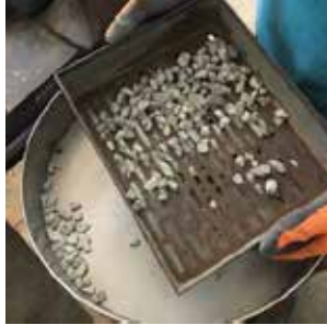
Figure 2: (a) Determination of flakiness index,
