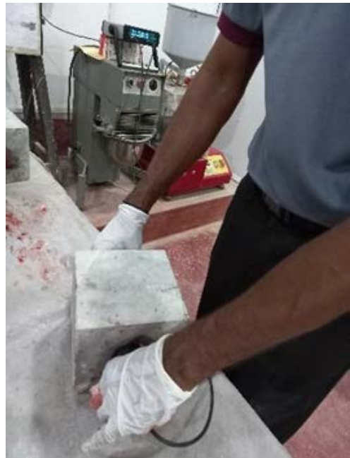
Figure 1: UPV testing for concrete cubes (UPV test was carried out in accordance with BS EN 12504-4:2004)
