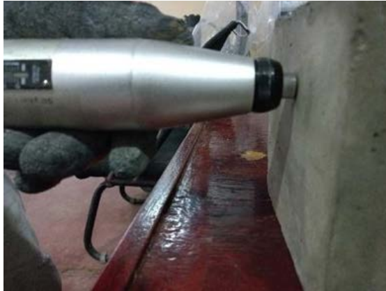
Figure 2: Picture showing the RH Testing of representative concrete cube
