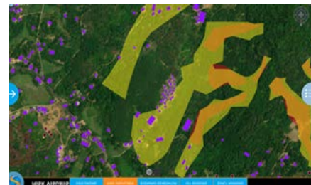
d) Landslide flow path simulation: The landslide flow path simulation was derived based on the Yellow/Red zoning concept. The yellow zone represents the low-impacted areas, and the red zone the high-impact areas.
