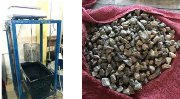
Figure 1: (a) specific gravity frame, (b) SSD aggregate sample
