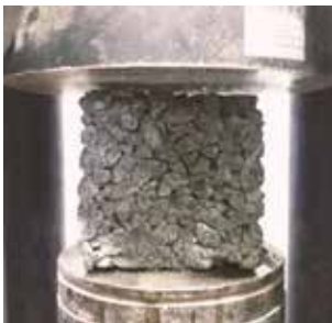
Figure 3: Test for compressive & flexural strength
