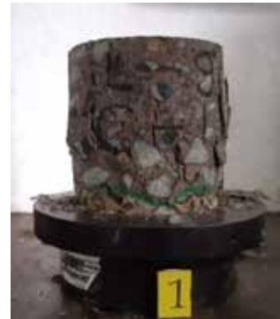
Figure 11: Failure after compressive strength test, School ID-K
