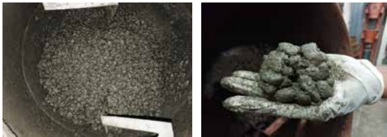
Figure 5: Pervious concrete mixture
