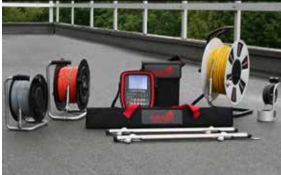
Figure 5: Inclinometer monitoring apparatus
