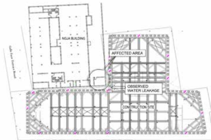
Figure 2: Plan view of the leakage point and the damaged location [2]
