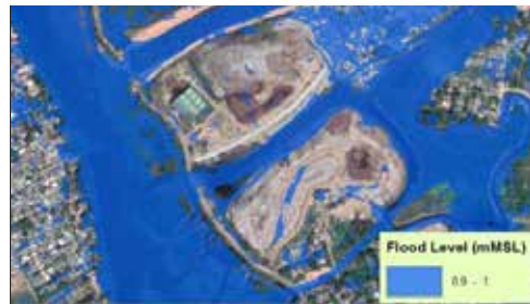
Figure 09: Flood Spread Map for 05 Year Return Period for raw terrain with dredged canals [Future Condition]
