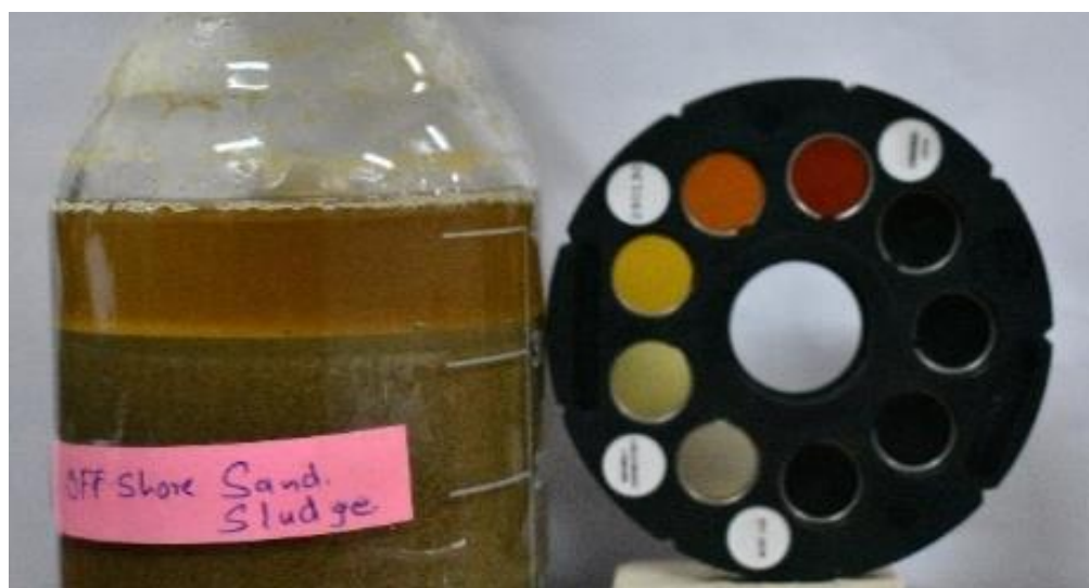
Figure 02: Supernatant color comparison with standard color plate according to ASTM C40
