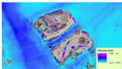
Figure 14: Flood Velocity Map for 100 Year Return Period for raw terrain without dredged canals [Present Condition]
