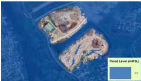
Figure 08: Flood Spread Map for 5 Year Return Period for raw terrain without dredged canals [Present Condition]
