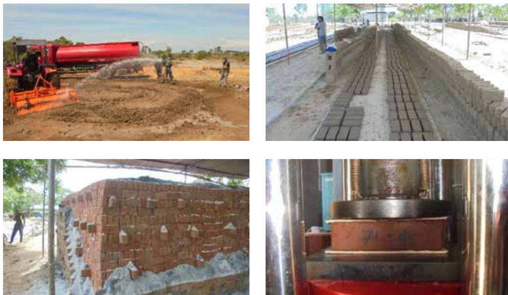
Figure 01: Brick making process and the test for compressive strength
