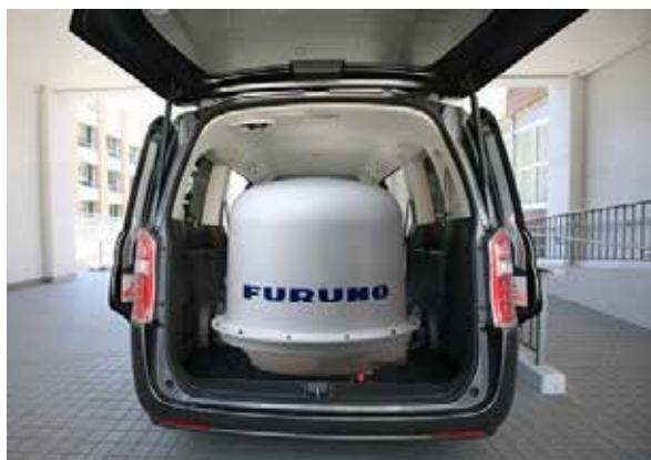
Figure 01: X-band dual polarization weather radar carried by a vehicle
