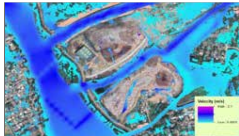
Figure 11: Flood Velocity Map for 5 Year Return Period for raw terrain with dredged canals [Future Condition]
