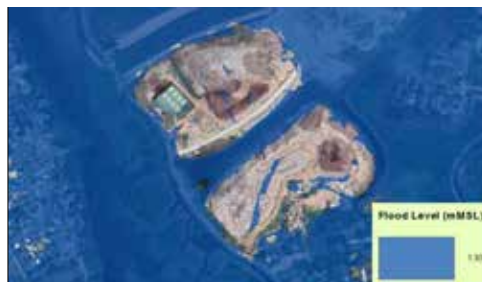
Figure 13: Flood Spread Map for 100 Year Return Period for raw terrain with dredged canals [Future Condition]
