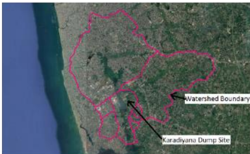
Figure 04: Catchment delineation for the Karadiyana dumpsite area
