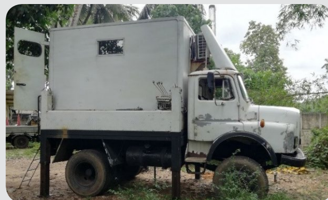
Fig. 1. Truck mounted CPT rig
